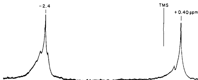
Figure 1. ^1\text{H} nmr spectrum of \text{Al}_3(\text{CH}_3)_3[\text{N}(\text{CH}_3)_2]_2 .
